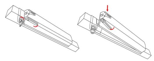
To put the battery back into place, insert the battery along to the guide rail. Push it closely against the controller box. Click in place to fasten the battery lock.
