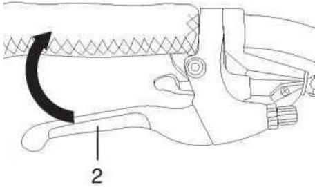
The right brake lever (2) controls the rear wheel
