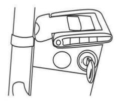
The 3 green LEDs located on top of the battery indicate its charge level.
