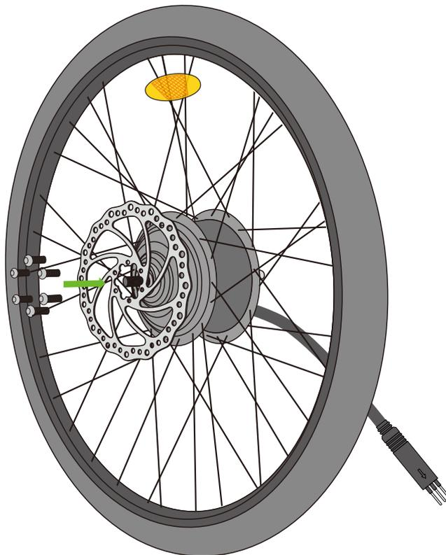
2.3. Fix disc brake first, then twist screw. (pay attention to disc brake pad direction)
