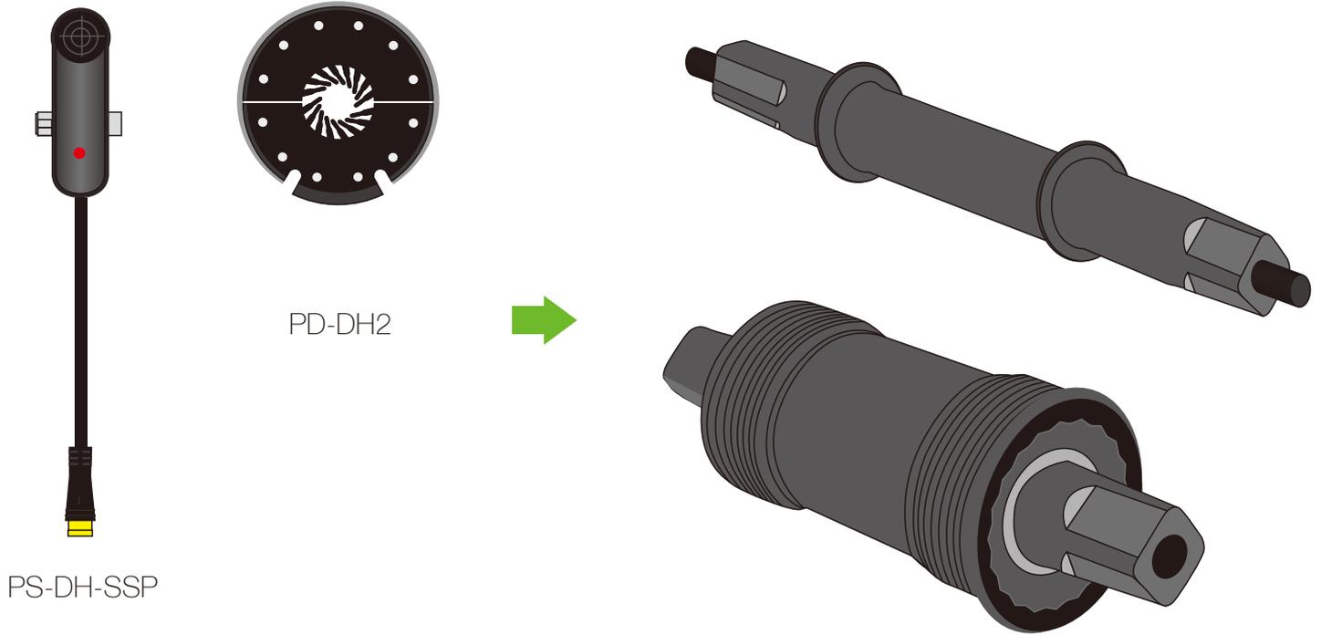
PAS sensor&PAS disc should be assembled on left side of the 2 kinds of bottom bracket.
