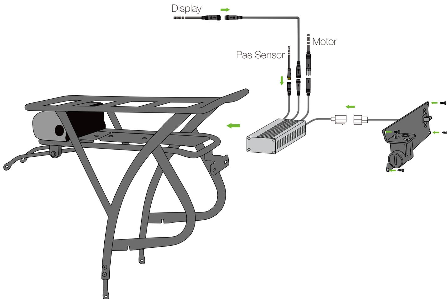
3.1 Connect controller with motor, display, PAS Sensor, battery. Put controller into the controller case.
