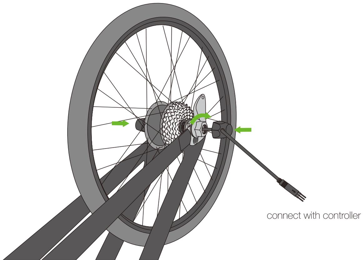
2.7. Fix motor wheel, fasten the nut, cover with axle cap and make the motor cable connect with controller.
