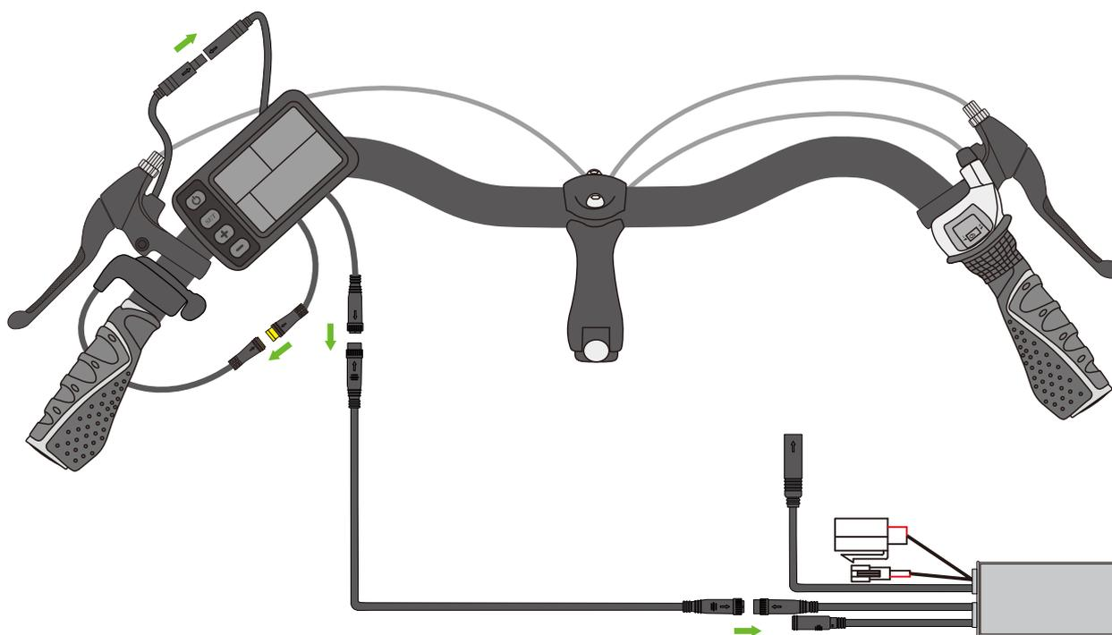
4.2 Instal brake cable and throttle cable, connect E-brake lever and throttle with display, connect display cable with display extension cable, and then connect with controller.
