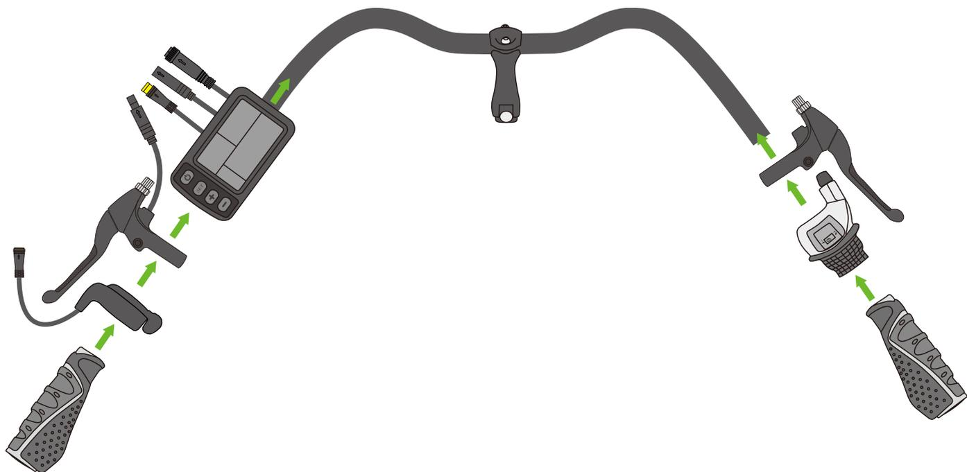
4.1 Take off the original grip and brake lever, assemble the display, brake lever set, thumb shift throttle in turn from kits, and then instal grip.
