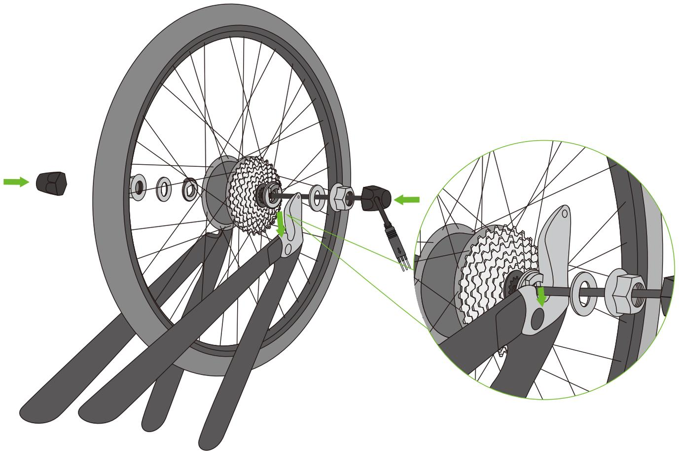
2.6. Please pay attention to wheel installing direction after assembling rear wheel according to the sequence in the picture above.
