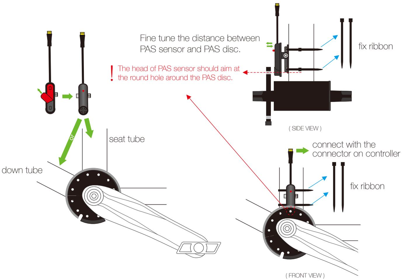
1.2.2. Assemble PAS sensor and fix with ribbon.
