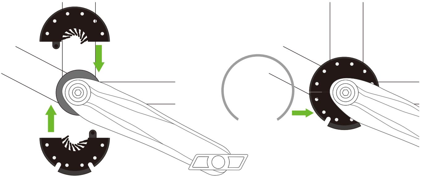
1.2.1. Assemble PAS disc, fasten metal ring to fix it.
