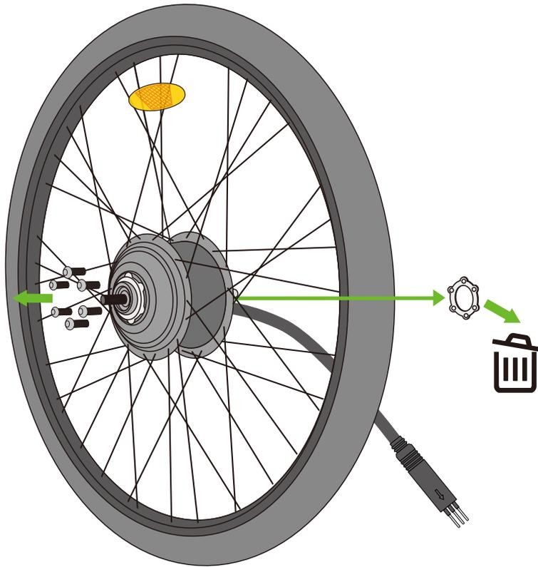
2.2. Remove screws and shim from motor.
