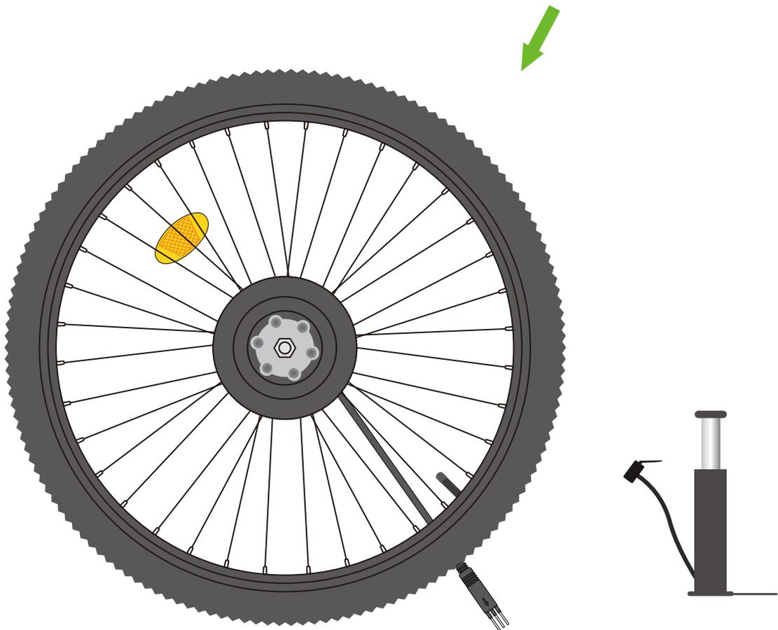
2.1. Assemble inner tube & tire on motor wheel and pump up
