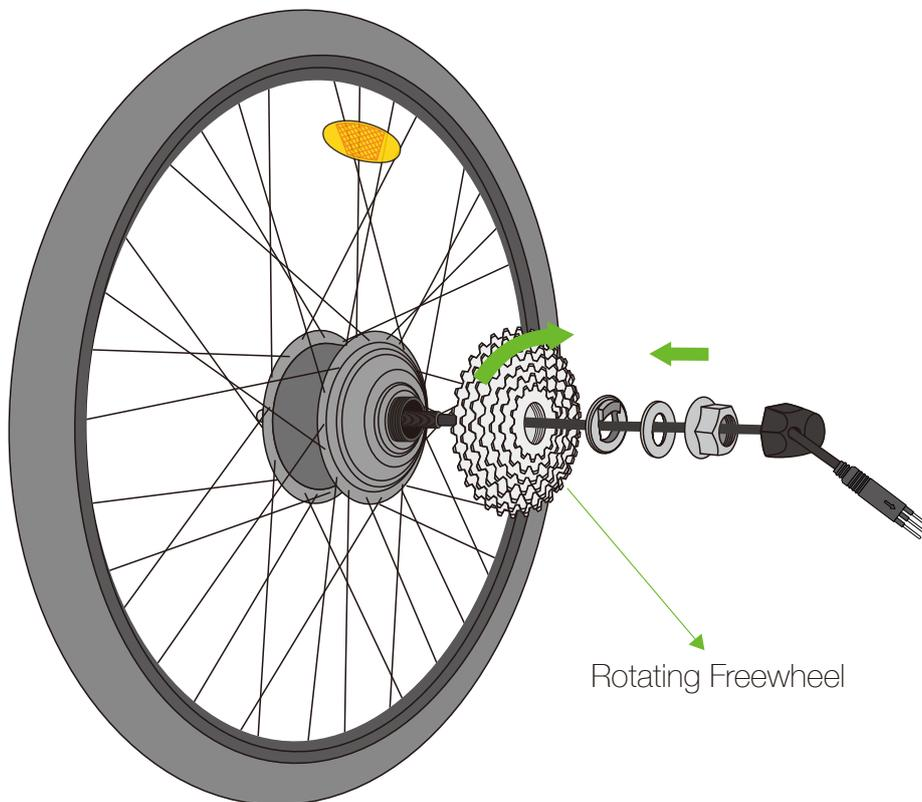
2.5. Please assemble fix rotating freewheel according to the sequence in the picture above.
