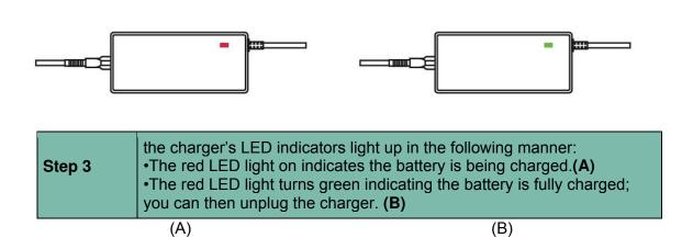
When depleted, it takes 6.5 hours for the battery to completely recharge using the standard charger supplied with the bike.
