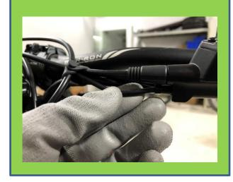
Step 2: remove the ignition key switch cap, find the sensor plug and disconnect the plug. Put the bike on the stand, lift the side stand, test the bike, if the motor back to work, then we can confirm the brake power protection malfunction, replace new part to repair.
